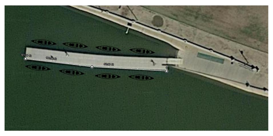
The dock is ~120 ft long on both sides, and nearly level to the water. Assuming each boat is 22 ft long, and requires a few feet of buffer space, the dock can handle 8 boats at once.
